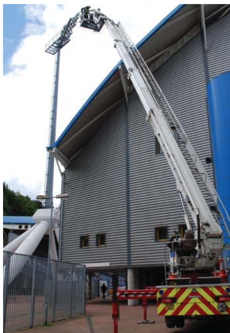
Aerial platform with wireless camera capable of transmitting live imagery back to fire and rescue command vehicle.
